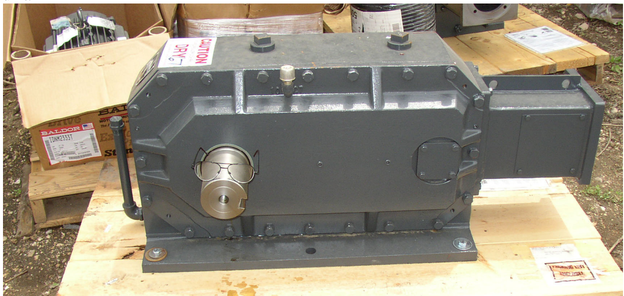
Photo 5: The Work Horse- Gearbox Note Eyeglasses- 5.25" Output Shaft
