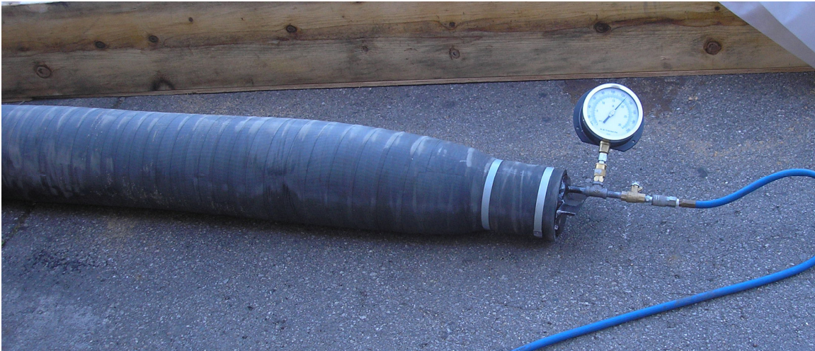
Test section under 18 psi load.
